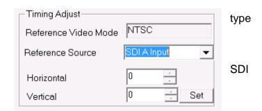
**Vertical** adjusts the relative vertical timing between the Genlock signal and the cards output signals.
