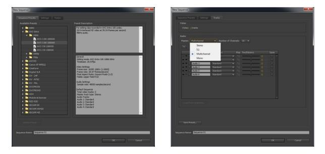
To output up to 16 channels of embedded SDI audio with 8 channels of AES select *Multichannel* from the *Master* selection of the *Tracks* tab. The Adobe audio mixer will now allow you to send audio to the appropriate Bluefish444 audio channels, 1-16.
