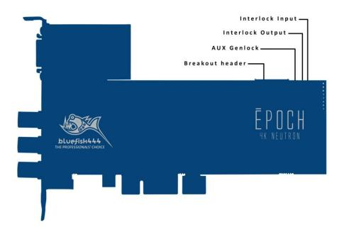
Multiple Neutron cards may be locked together sharing a common clock. This is achieved by attaching the *Interlock cable* (Part Number CAB\_ILOK) from the *Interlock Output* of one card to the *Interlock Input* of a second card.
