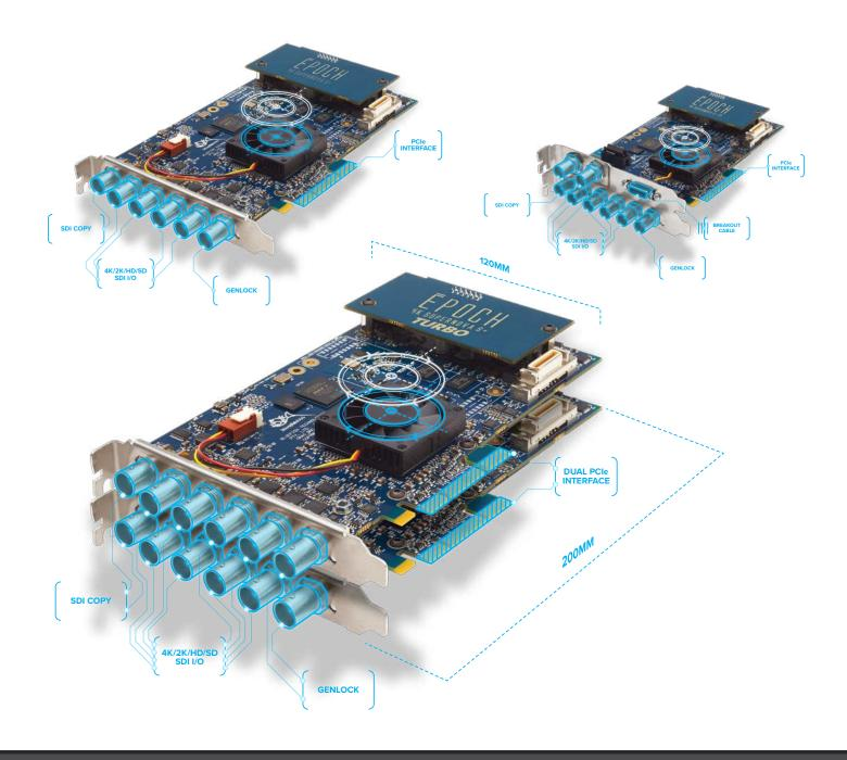
THE WORLD'S FIRST 4K CAPABLE SDI VIDEO CARD RANGE WITH BI-DIRECTIONAL BNC'S PROVIDING UP TO 4K 60P CAPTURE AND PLAYBACK
